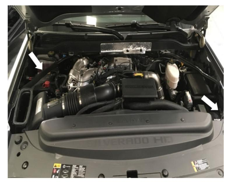
With the ignition switched off and the parking brake set, disconnect the negative battery cables on both batteries.
