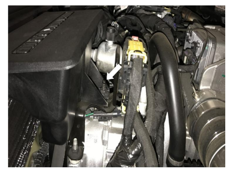
Remove the nut securing the stock resonator.
