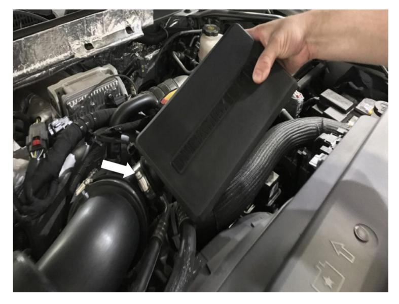
Loosen the hose clamp at the resonator then remove the resonator from the intake tube.
