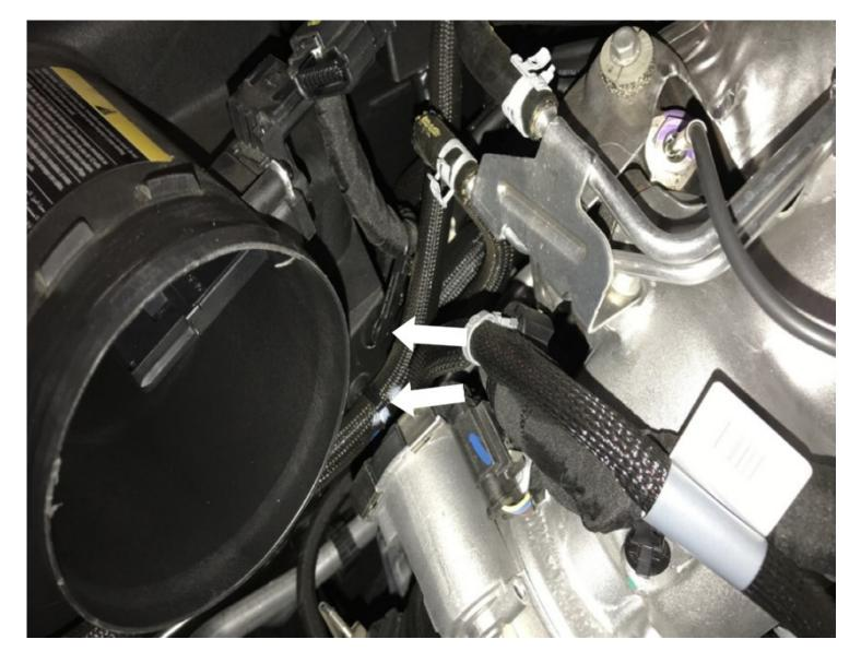
Disconnect the two black clips securing the MAF electrical harness to the intake box.
