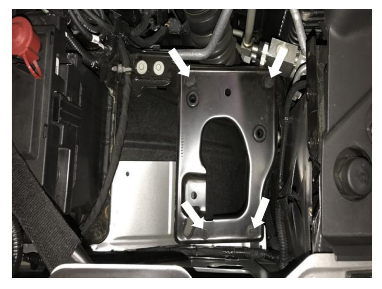
Remove the four bolts securing the intake box tray, then remove the tray from the vehicle.
