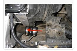
11. Place one the supplied T-bolt Clamp (I) over the Straight Coupler (H) and slide it on the upper end (Large diameter) of the Boost Tube (J).
