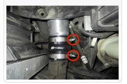
**16.** Install the other O-Ring (B) in the top groove of the Billet Spacer Block (A). Insert the S&B Intake Elbow (C) into the Straight Coupler (H) and align the mounting holes with the Billet spacer. Be sure both mating
