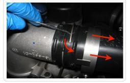
7. Apply sealant (Teflon tape) to each 1/8"NPT Plug (G) and insert the plugs into the ports you will not use on the elbow. Use 3/16" Hex drive and torque the plugs to 40 ln.lbs.
