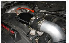
$19. \ \text{Reinstall the Intake or OE air cleaner} \\ \text{and filter removed in Step 3.} \\$
