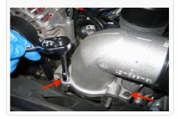
**9.** Remove the other clamp from the OE boost tube. Clean the two clamps as they will both be re-used on the lower connection of the new tube.
