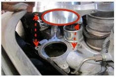
18. Position the upper T-bolt clamps as to not hit the hood when closed and torque them both to 50 In.lbs.
