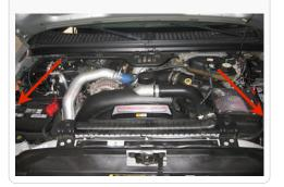
4. Loosen the upper hose clamp at the OE elbow and pry the compression clip out of the groove.
