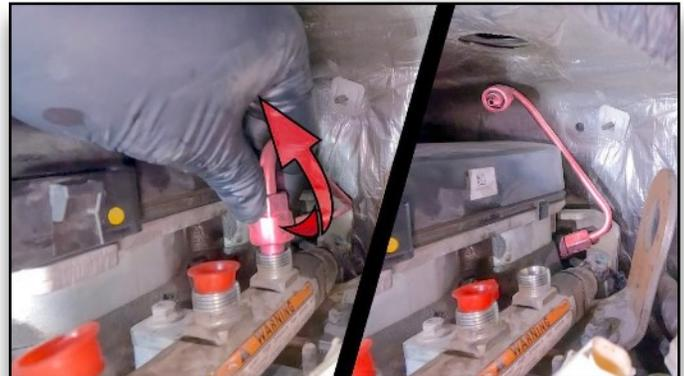
**56. Loosen #6 Fuel Line, Rotate Out of Way**
