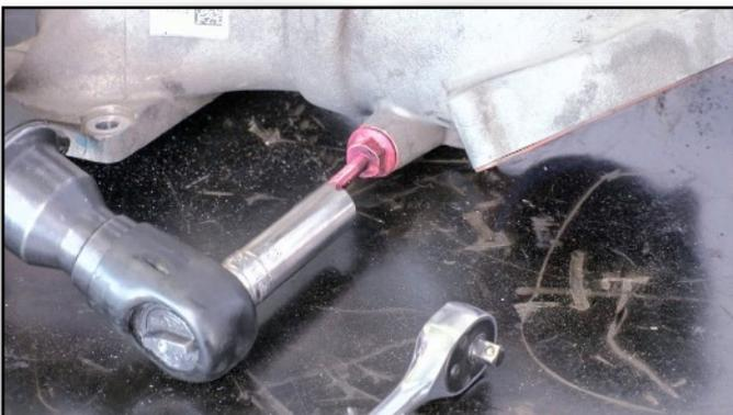
**71. Remove & Transfer Elbow Stud**
