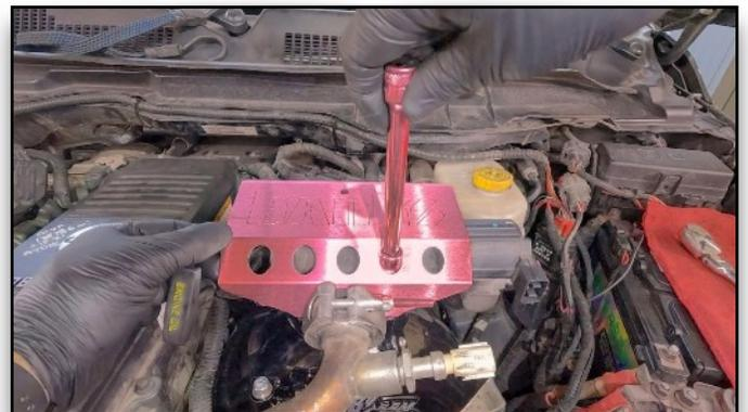
**125. Install EGR Heat Shield & Tighten Bolts**
