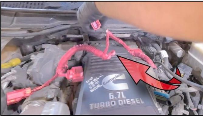
**96. Route Engine Harness Under Dipstick & Around Valve Cover**
