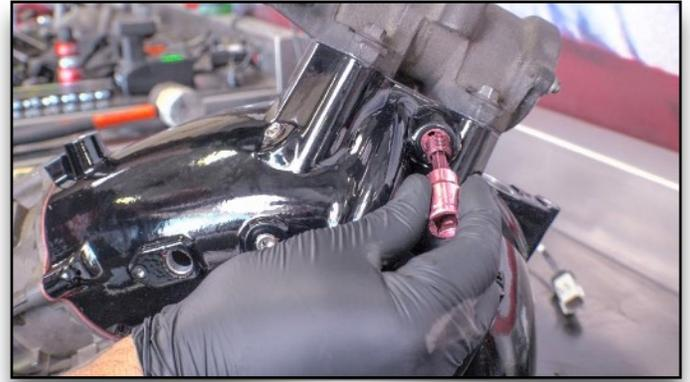
**78. Install Rear Thermocouple Plug**
