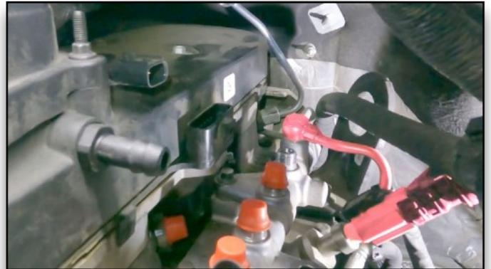
**85. Re-Install Temp Sensor. Hand Tighten Washer & Banjo Bolt**
