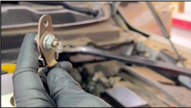
**114. Assemble Heater Cable Extension Bracket**
