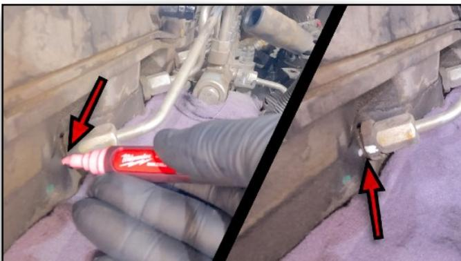
**53. Paint Marker Line Across Threaded Insert & Cylinder head**
