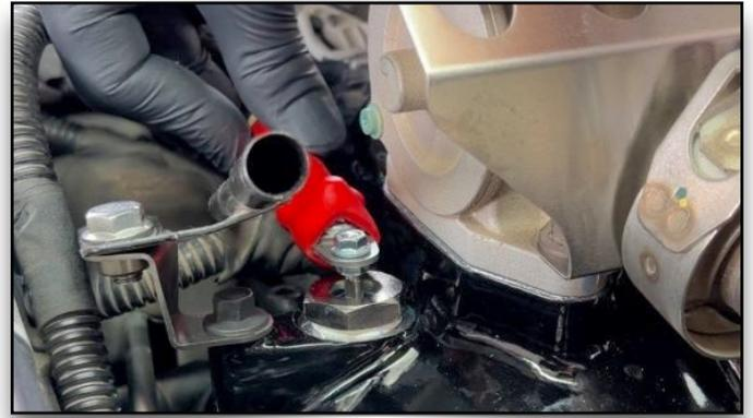
**116. Place Heater Cable Onto Threaded Post**
