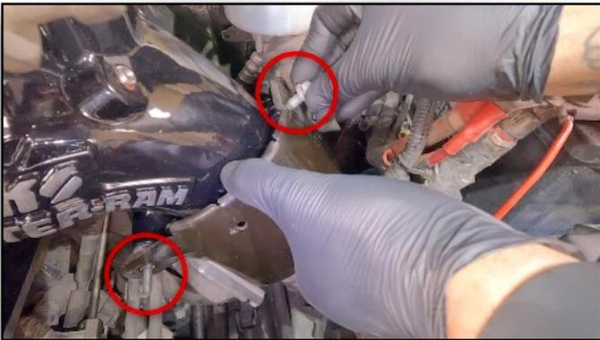
**128. Install Throttle Heat Shield Bolt & Nuts**
