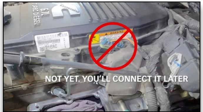
**99. Do Not Connect Front Blue Injector Plug Yet**
