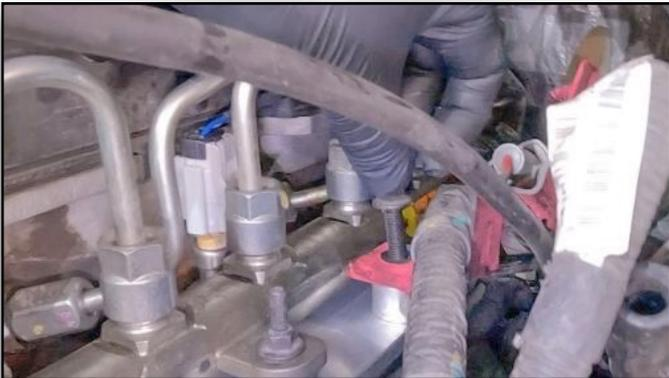
**Slide Dipstick Bracket Over & Reinstall Stud**
