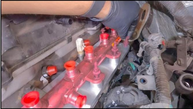
**83. Release Bungee Cord. Place Fuel Rail & Studs in Place**
