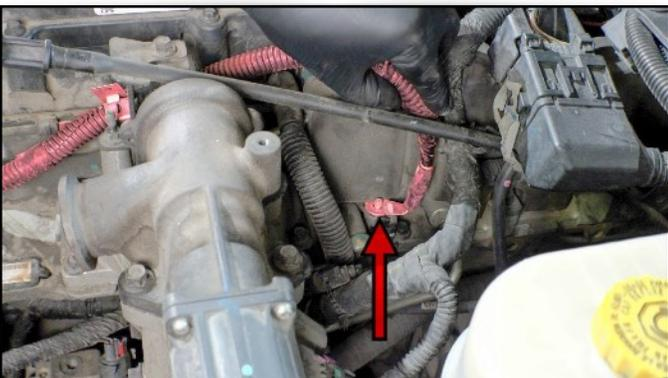
**29. Remove Heater cable from Terminal**
