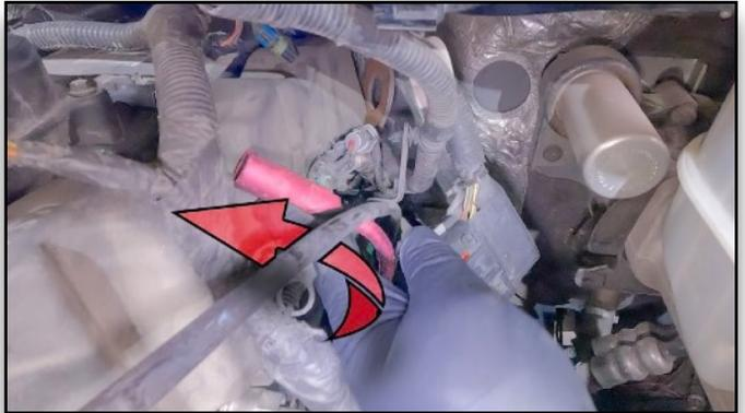
**92. Run Rear RCV Hose Under Dipstick Tube**
