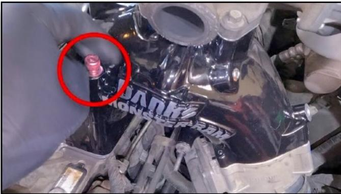
**102. Put Long Bolt Into Front Corner by Hand**
