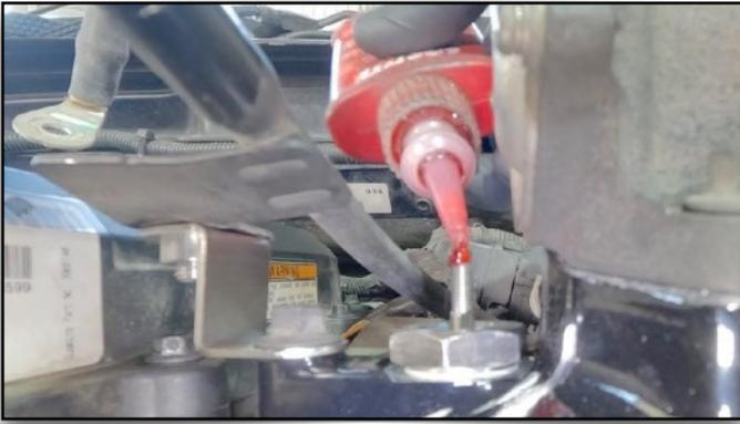
**113. Apply Red Thread Locker to Coil Heater**
