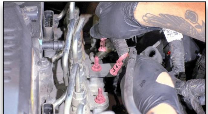
49. Remove Cable Ties from Driver Side Studs
