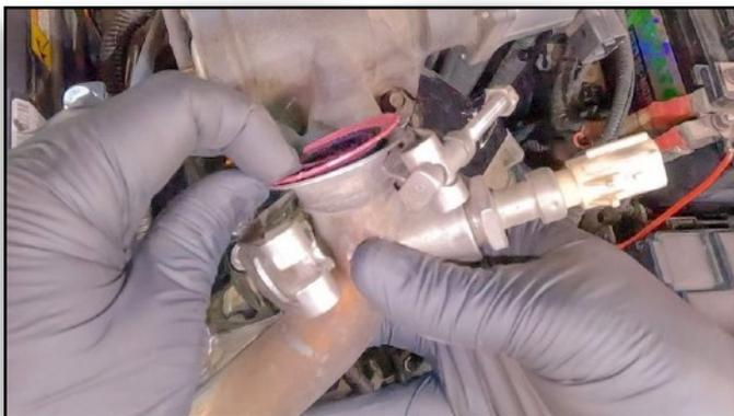
**121. Conical Gasket Goes On Driver Side of EGR Tube**
