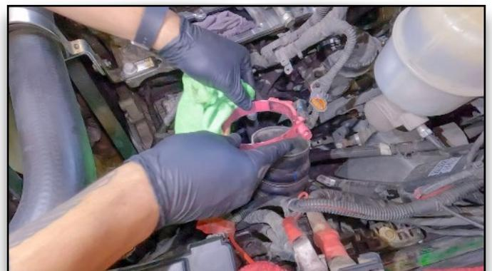
**100. Remove Rag From Boost Tube, Put Clamp Back On**
