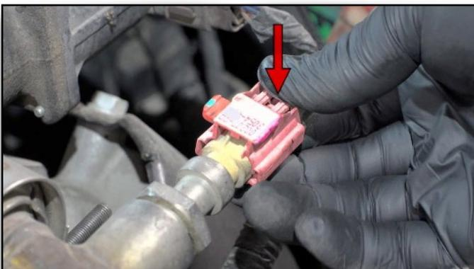
**17. Remove Temp Sensor by Pinching It**
