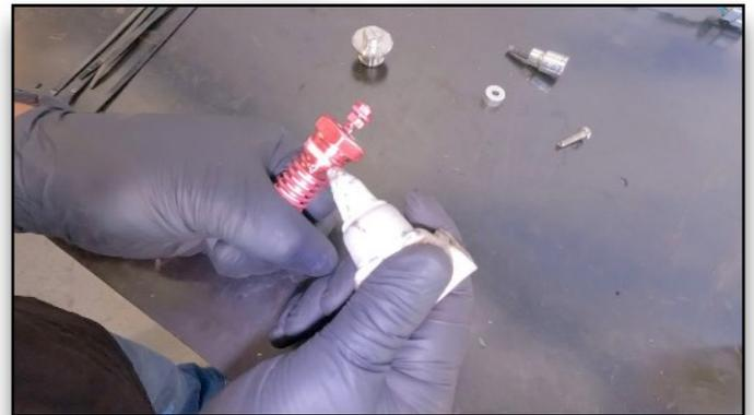
**104. Apply Sealant To Heater Coil**
