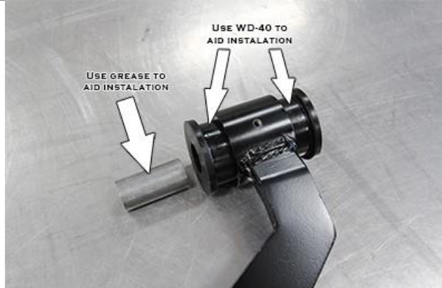
Figure 3: bushing and crush sleeve installation
