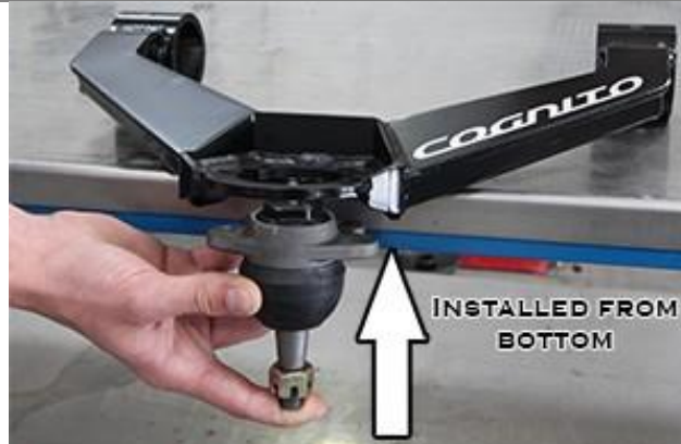
Figure 2: ball joint installation
