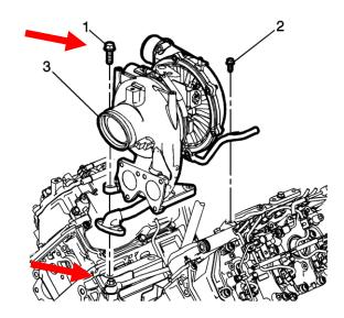
32. Install the turbo oil return tube fasteners (1) and tighten to 18 ft lbs.
