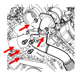
20. Remove the left exhaust pipe to turbocharger upper bolts. Remove the left exhaust pipe.
