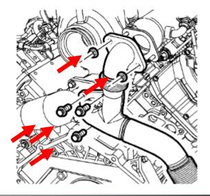
39. Install the exhaust outlet and tighten the exhaust outlet clamp. Torque to 11 ft lbs.
