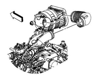
10. Loosen the air intake pipe to turbocharger clamp and remove the air intake pipe from the turbocharger. The clamp will be reused.
