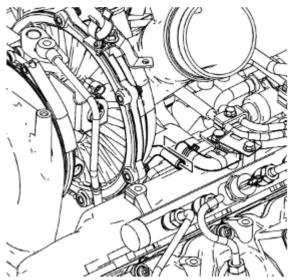
42. Install the turbocharger outlet coolant hose to the turbocharger and position the hose clamp. Install the turbocharger inlet coolant hose to the turbocharger coolant bypass valve.
