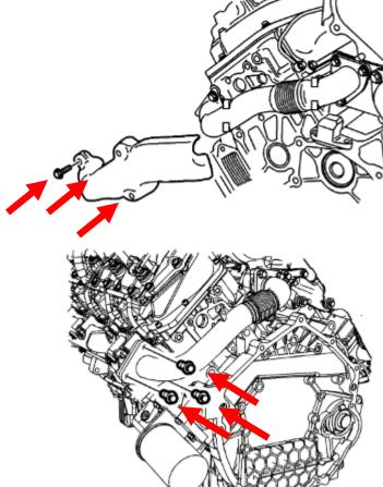
6. Remove the right side exhaust pipe to exhaust manifold lower bolts only.
