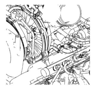
15. Remove the turbocharger upper heat shield bolts and remove the turbocharger upper heat shield.
