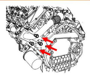
51. Install the left side heat shield and heat shield bolts. Torque to 71 in lbs.
