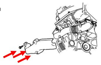
52. Slide the clamp back up onto the exhaust pipe. Tighten the clamp to 11 ft lbs.
