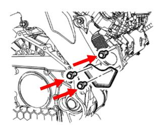
50. Install the left side exhaust pipe to exhaust pipe to exhaust manifold bolts. Torque to 39 ft lbs.
