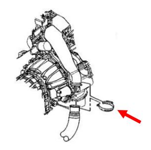
4. Remove the left side exhaust pipe heat shield bolts and remove the heat shield.
