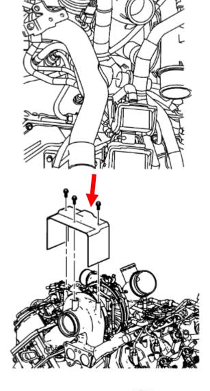
44. Install the charged air cooler inlet duct connector (4) to the turbocharger. Tighten the charged air cooler inlet duct connector to turbocharger clamps (1, 3). Tighten the clamps to 53 in lbs.
