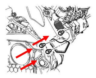
7. Remove the lower bolt for the right side exhaust outlet shield.
