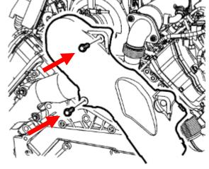
41. Install the PCV hose/pipe. Install the turbocharger outlet coolant pipe banjo bolt and washers.
