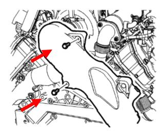
16. Remove the remaining exhaust outlet heat shield upper bolts and remove the exhaust heat shield.
