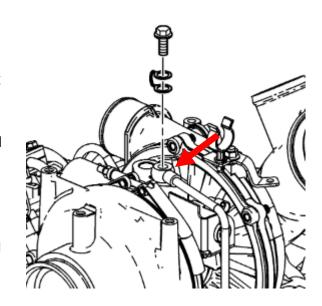
36. Install the left side exhaust pipe and a new uppipe gasket (item 3) included in the kit. Torque the bolts to 39 ft lbs.
