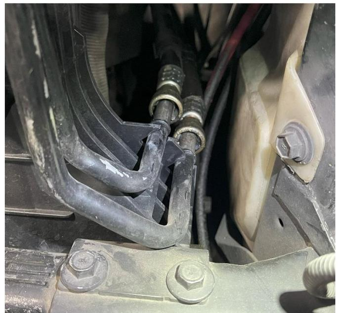
**STEP 5:** Using a ½" quick disconnect tool, disconnect both lines routed on the driver's side of the transmission cooler.
