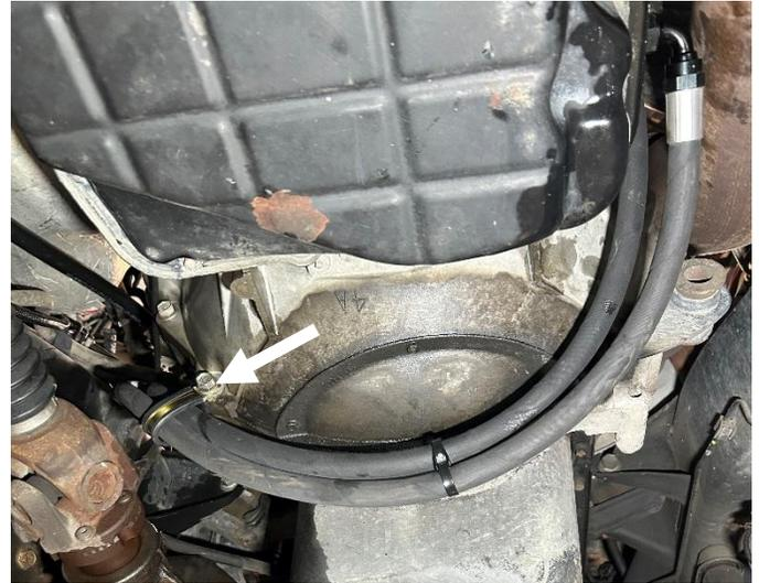
**STEP 18:** With the cooler lines routed and retained, tighten each of the four cooler line fittings to 270-350 in-lbs using a 1" wrench. Use a backup wrench on the AN adapters installed in the housings of the transmission cooler and transmission to prevent overtightening.
