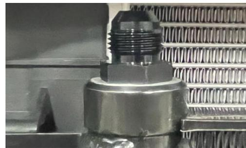
**STEP 12:** Install the 90-degree fitting of the long transmission cooler line onto the passenger side port of the transmission cooler using a 1" wrench. Do not tighten the fitting. Route the line parallel to the top of the transmission cooler assembly.
