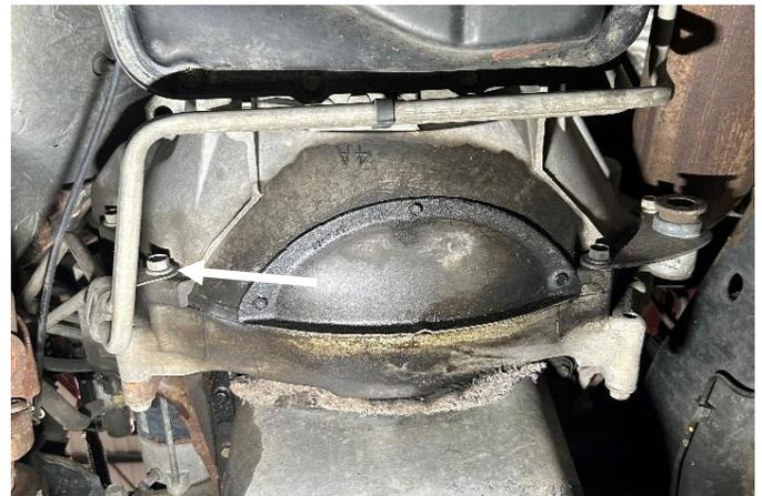
**STEP 8:** Remove the c-clips from the transmission cooler line fittings on the transmission. Remove the OE transmission cooler lines from the vehicle.
