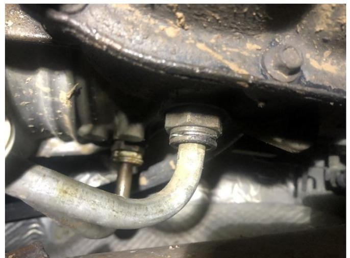
**STEP 9:** Use a 1" wrench to remove the factory fittings from the transmission and replace them with the -8AN to 3/4"-16 fittings.
