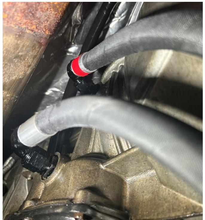
**STEP 16:** Install the included double hose clamp onto the transmission bellhousing using a 14mm socket or wrench.
