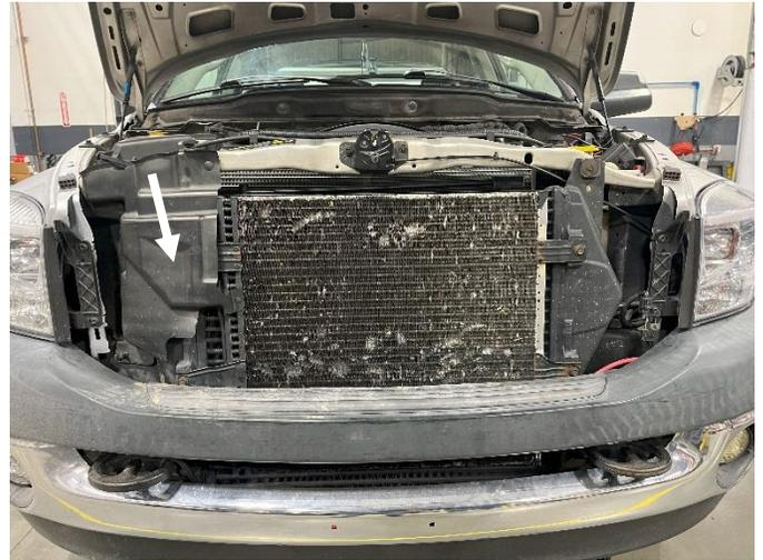
**STEP 3:** Remove the four bolts retaining the AC condenser to the front of the intercooler using a 13mm wrench or socket. Rest the condenser on the front bumper and use painter's tape to protect the bumper.
