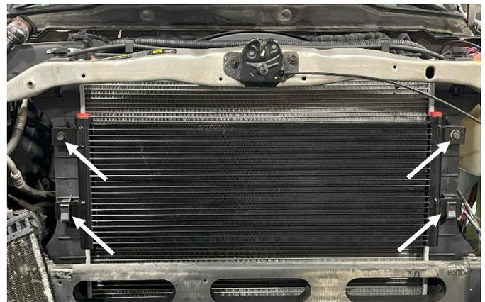
**STEP 11:** Remove the red caps over the ports on the transmission cooler and install the two fittings into the assembly using a 7/8" wrench. Tighten the fittings to 22 ft-lbs.
