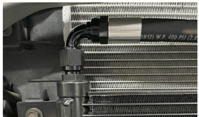
**STEP 13:** Install the 120-degree fitting on the short transmission cooler line onto the driver's side port of the transmission cooler using a 1" wrench. Do not tighten the fitting.
