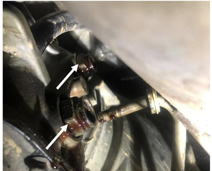
**STEP 10:** Install the new Fleece Performance transmission cooler assembly. Insert the two tabs into the slots, then use a 13mm wrench or socket to install the two bolts retaining the cooler.
