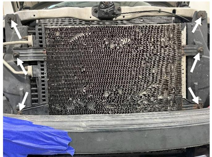
**STEP 3:** Loosen the hose clamps on both sides of the intercooler using an 11mm socket or wrench. Remove the two bolts retaining the intercooler to the frame using a 10mm socket or wrench. Remove the intercooler.
