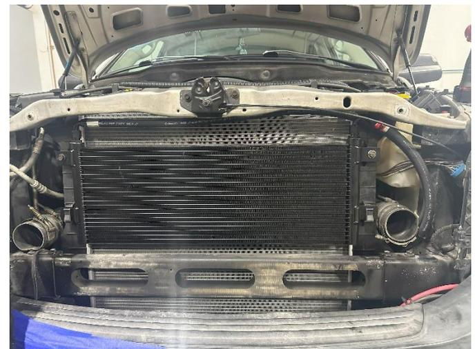
**STEP 20:** Install the intercooler and tighten the charge tube clamps using an 11mm socket or wrench. Install the two bolts that retain the intercooler using a 10mm socket or wrench.
