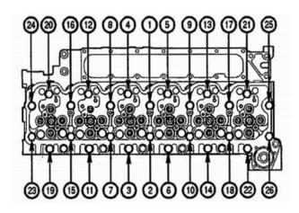
**STEP 8:** Lubricate the tops of the valves and re-install the OEM rocker bridges with the indicating marks (dots) facing the exhaust side OR install Fleece Performance rocker bridges (FPE-BRAB-C1).
