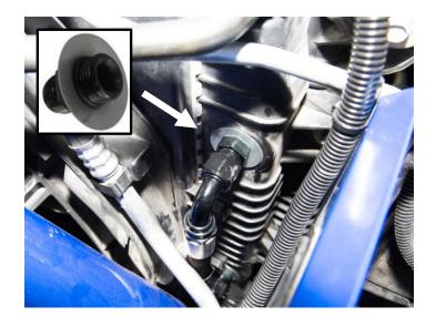
Remove the two OE fittings from the transmission using a 1 ½" socket or wrench.
