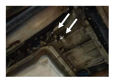
Install two of the 7/8"-14 O-ring to -10AN fittings into the "To Cooler" and "From Cooler" ports on the transmission.
