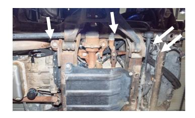
The shortest length line is routed from the transmission "TO COOLER" to the bottom-side radiator fitting. The 45 degree fitting is utilized on the radiator side, aligned slightly downward and toward the center of the chassis.
