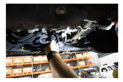
Remove the lower supports for the front bumper from the left and right sides of the vehicle.
