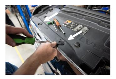
Remove the front grill retention bolts located along the top of the grill.
