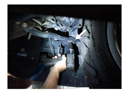
Remove the front bumper assembly to provide for clear access to the transmission oil cooler.
