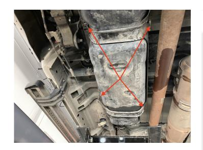
Lower the tank approximately 6" or until you can reach the electrical connector, feed line, and return line on the fuel sending unit.
