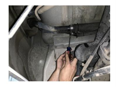
Remove the OEM skid plate if equipped. This will not be used again.
