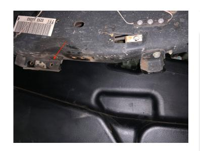
Center the hydraulic jack underneath the fuel tank and raise until the jack contacts the tank. Caution: Support the tank properly as remaining fuel can slosh and cause the tank to shift.
