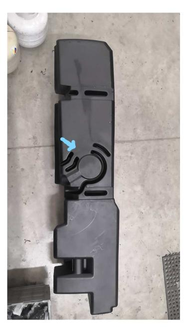
Raise the vehicle up on a lift to working height. The rear of the driver's side frame rail needs to be unobstructed as the S&B Tank will protrude under the frame rail.
