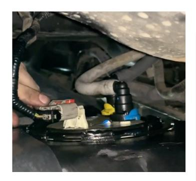
Disconnect the fuel feed & return lines. The base of each connector has a lock. Pull the lock away from the center of the connector, depress the yellow or blue tab, press down and then pull up on the connector. Be patient with this step as these connectors are fragile and can break.
