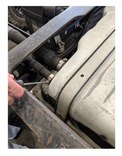
Center the hydraulic jack underneath the fuel tank and raise until the jack contacts the tank. Caution: Support the tank properly as remaining fuel can slosh and cause the tank to shift.
