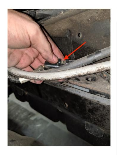
Remove both the feed and return lines from the sending unit. Squeeze the blue buttons on the fuel connecter, gently press in towards the barb then pull off.
