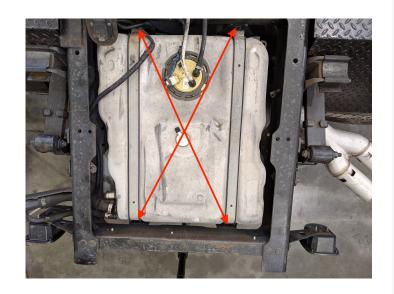
Lower the tank 6" until you can easily reach the fuel sending unit to disconnect all connectors.
