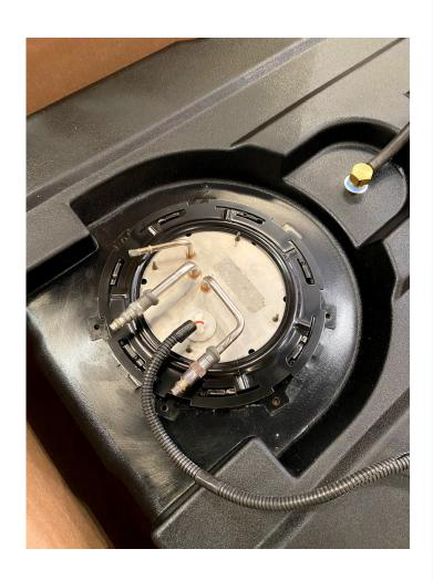
On the OEM fuel tank. Use a 19 metric socket to remove 2 strap bolts which hold the stock fuel tank into the skid plate.
