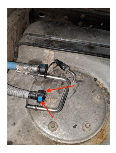
Now the tank is completely disconnected from the vehicle and can be lowered from the vehicle. Ensure the tank is still properly supported as remaining fuel can slosh and cause the tank to move.
