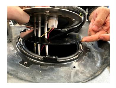
Place the S&B locking ring over the sending unit and hit the ring clockwise until the rib on the OEM locking ring is fully seated past the indentation on the S&B receiving ring.
