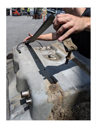
Place the S&B Tank in the OEM skid plate, reassemble the straps using a 19mm socket.
