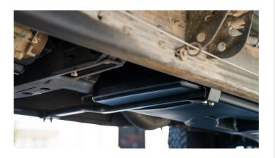
To secure the S&B support bar to the frame. Slide the ubolts over the bar and slide as close to the frame as possible. Then install the clips, washers and lock nuts onto the u-bolt. The larger of the 2 clips goes onto the driver side frame.
