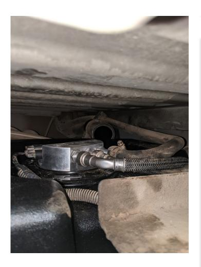
Reconnect the 2 fuel lines coming from the sending unit onto the fuel cooler.
