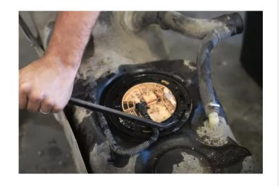
Place the S&B o'ring into the o'ring groove then drop the sending unit into the tank.
