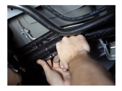
Release the DEF lines from the bracket on the OEM tank
