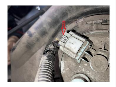
Hit the locking ring counter clockwise to release the OEM sending unit.
