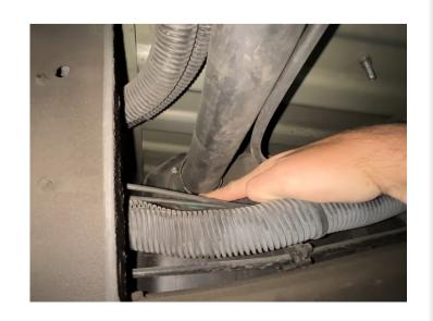
Remove the hose clamp and hose from the main vent line attached to the fuel sending unit. You can reach over the driveline to access this.
