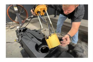
The tab on the sending unit should face the skinny arrow on 2017-19 trucks and the block arrow on 2011-16 trucks
