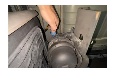
Remove both fuel tank straps with a 15mm socket.
