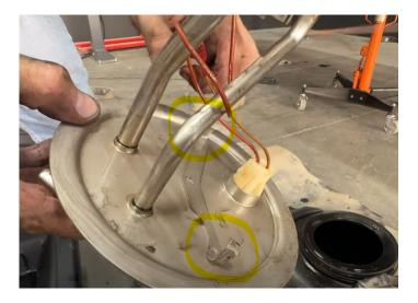
Place the sending unit into the S&B Tank with the larger fuel nipple perpendicular to the fuel tank. Reuse the OEM locking ring and tighten.
