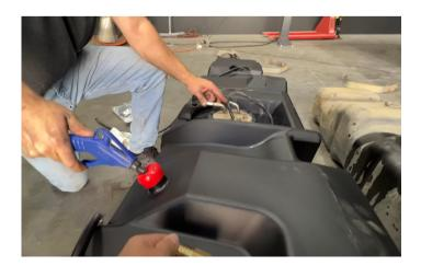
Remove the filler and vent hose from the OEM tank and transfer to the S&B Tank. Before putting the filler on the S&B Tank, put the included check valve into the end of the hose that will be connected to the tank. The flow arrow should be pointing into the fuel tank.
