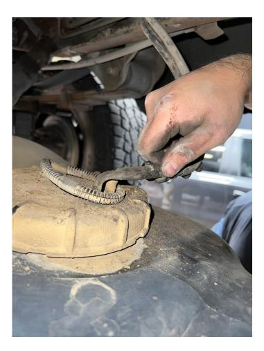
Remove the rubber rollover hose attached to the front and rear of the original tank.
