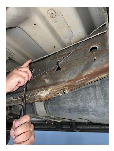
Remove the rear strap. The frame side bolt for the rear strap is right above the leaf string perch
