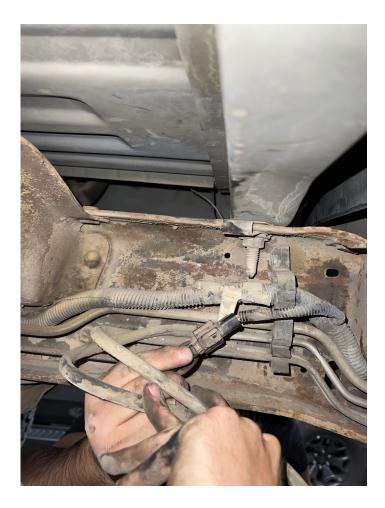
Press the buttons on the fuel lines and pull to remove both the feed and return lines.
