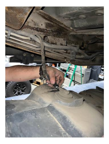
Use a dead blow and pry bar or large flat head screw driver to hit the locking ring counter clockwise. We will reuse this ring on the S&B Tank.
