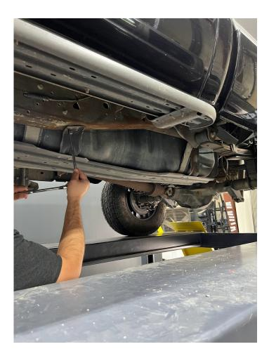
Support the bottom of the tank with a jack and remove the front strap. The bolt holding the front strap is on the outside of the frame.
