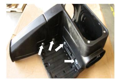
Install the Grommet into the side of the Airbox.
