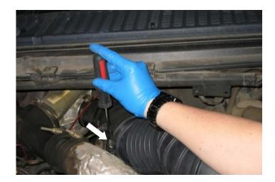
Unfasten and remove the stock airbox lid and intake tube assembly from the vehicle.
