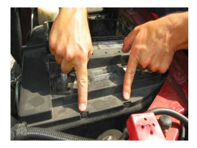
Remove the battery bolt and wedge then remove the battery from the vehicle.
