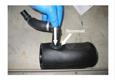
Insert the Short Tube (P) assembly into the Straight Coupler (R). Align the breather tube then secure using the #64 Hose Clamp (F).
