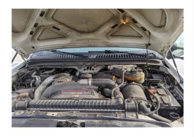
If Equipped: Disconnect the electrical connection at the OE restriction gauge located at the back of the airbox.
