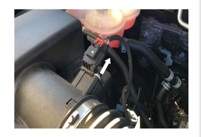
Remove the wire loom clip from the stock intake box lid.
