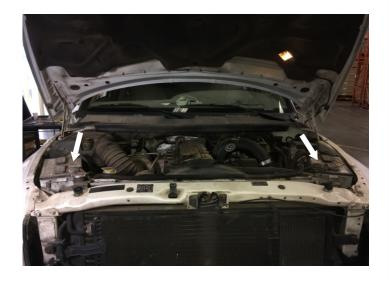
Use a Flat Blade Screwdriver or 5/16" Nut Driver to loosen the hose clamp at the turbo inlet. Then unclip the three clips on top of the airbox. Remove the stock airbox lid, air tube, and filter.
