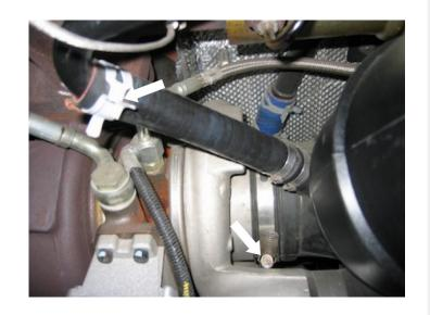
Remove the mounting nut on the core support securing the stock airbox.
