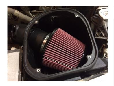
Reconnect the MAF and IAT electrical harness connectors. If necessary, zip ties the harness away from any engine components generating too much heat.
