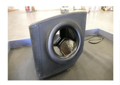
Install the Fender Seal (F) onto the Intake Box (A).
