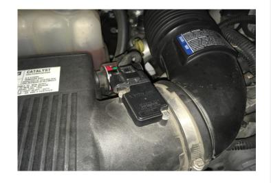
Remove the stock intake tube from the vehicle. Loosen the hose clamp at the turbo and stock intake box with a 5/16 Nut Driver or Flat Blade Screwdriver.
