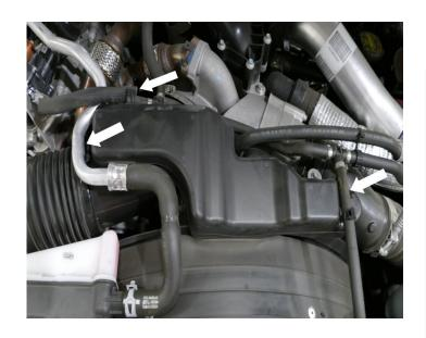
Remove the screw securing the air box to the battery tray. Set this screw aside, it will be reused in Step 14.
