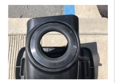
With this intake kit we have included a breakaway Box Plug (S) that is designed to keep engine heat out of your airbox but also serves as a safety mechanism that will protect your engine in the event that the main inlet of the intake becomes blocked with debris.
