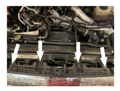
Pull the grill slightly forward and unclip the tabs securing the bottom of the grill to the vehicle. Then pull off the grill.
