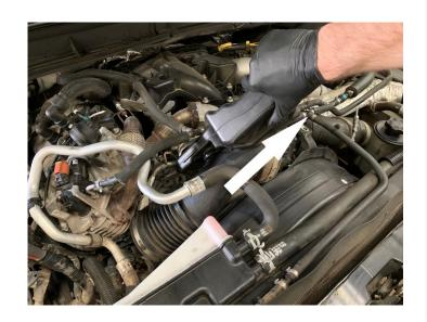
Remove the two screws securing the bracket under the airbox which holds the grommets to seat the airbox. Then remove the bracket from the vehicle. We will reuse one of the removed screws in step 10.
