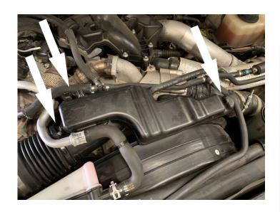
Lift the stock air box up to unseat the grommets from the air box tray and remove the stock air box from the vehicle.
