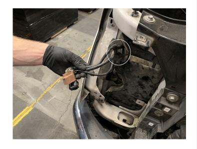
Disconnect the plastic air intake scoop from the frame of the vehicle by removing the series of plastic connectors found around the perimeter of the headlight opening.
