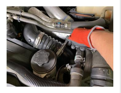
Using a Pick, locate the split in the Spring Clip and carefully remove the Spring Clip from the upper plastic CAC pipe.
