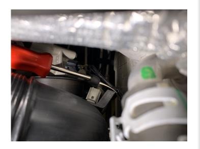
Loosen the lower hose clamp of the CAC outlet hose.
