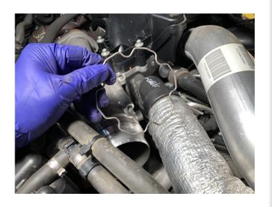
Remove the electrical connector from the Air Temperature Sensor located on the lower plastic CAC pipe. Depress the clip and pull it off.
