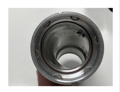
Add a thin coat of clean diesel engine oil around the outside diameter of the throttle assembly.
