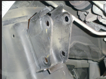
B. Modified idler support bracket for fitment of your new Death Grip Idler Support
