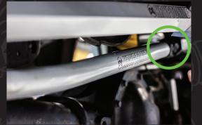
• Adjustment sleeve Jam nut torque - 185lb/ft
