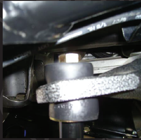
C. Bushings swell slightly when tightened properly, Do not over tighten!
