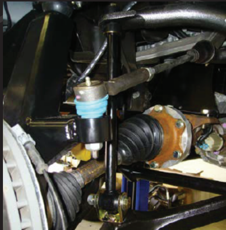
B. End Link in place, clevis rotated so bushing is relaxed.
