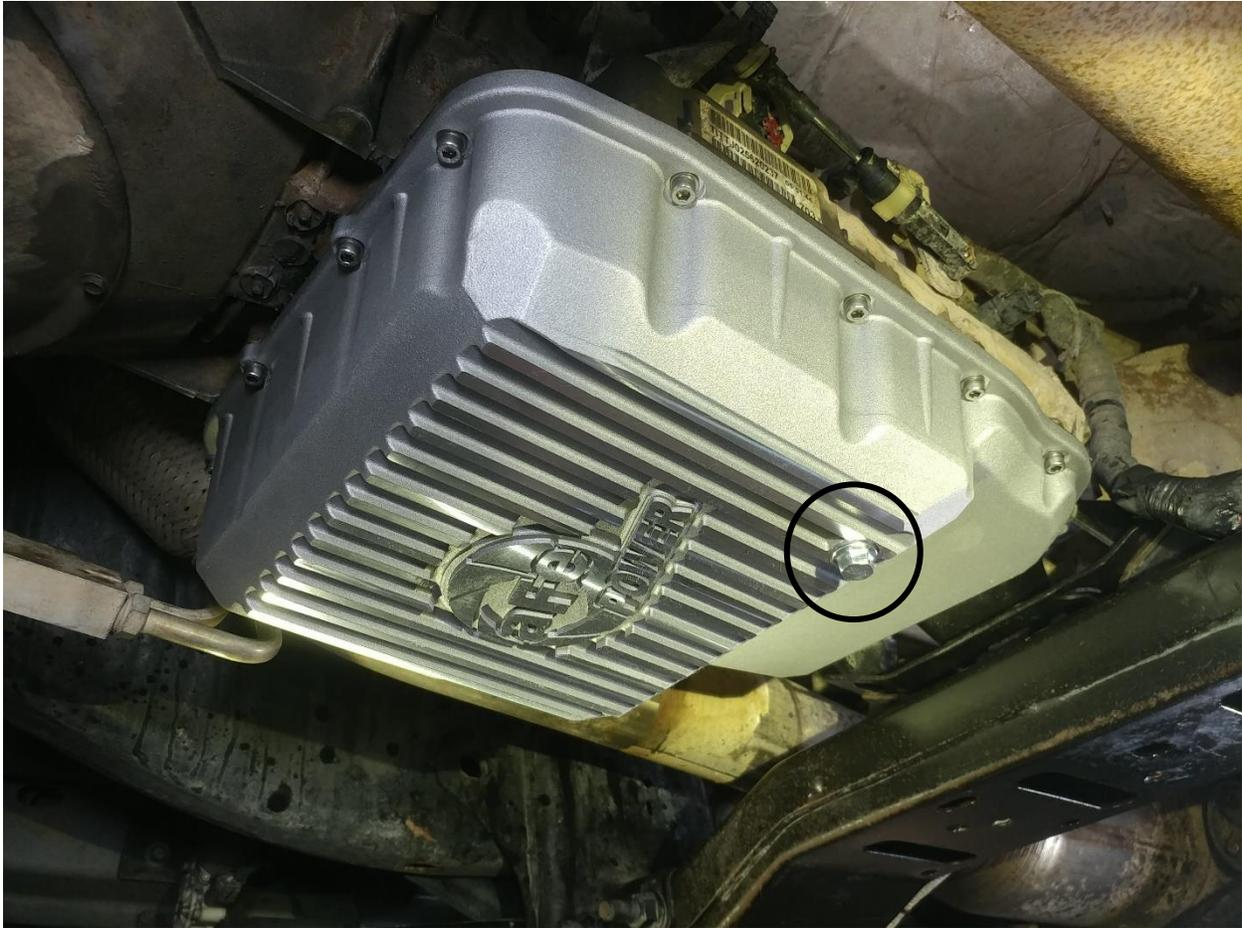
18. Install the supplied M12x1.25 magnetic drain plug and M12 crush washer into the bottom drain hole.
