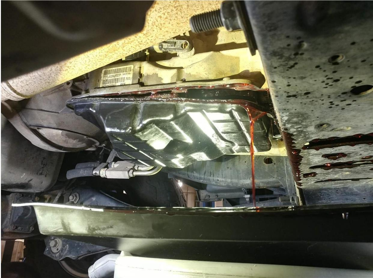
5. While positioned towards the front side of the pan, break the seal between the transmission pan and the transmission. The transmission fluid will begin to drain.
