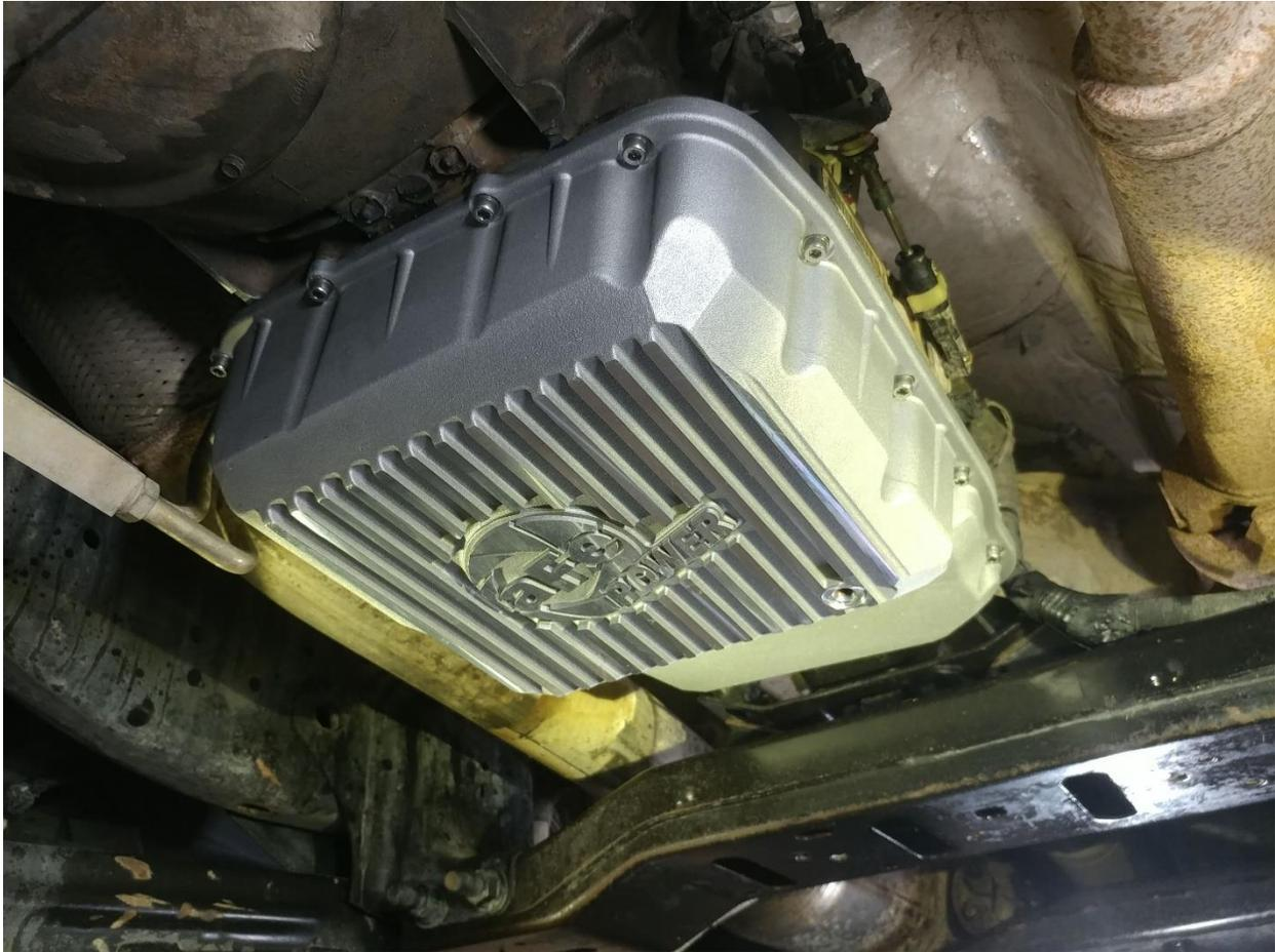
15. Hold the transmission pan up into position, aligning the screw holes. Install four (4) M6x1.0x20 socket head screws and M6 washers into each of the corners to hold the pan into place.
