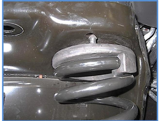
5. Lower the axle until you can slide the reservoir bracket between the rubber spring isolator and the upper spring mount.
