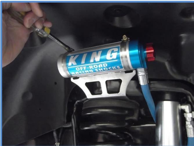
10. With the hose properly routed and the reservoir installed you can install and tighten the original lower shock bolt and tighten the upper nut.
