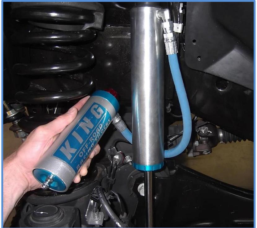
9. Mount the reservoir in the reservoir bracket using the supplied hose clamps.
